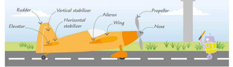
Elevators are flaps that vary the force of lift on the rear of the plane to pitch the aircraft's nose up or down. 2 Ailerons are flaps on the main wings. They move in opposite directions to make the plane roll, which helps it turn. 3 The rudder is an upright flap on the tail. Like a boat's rudder, it steers the plane, making it yaw (turn) left or right.
