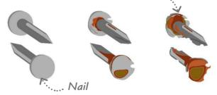
**2** Rusting Oxygen can react with many chemicals without causing fire. For example, iron and steel left in the air slowly react with oxygen to form iron oxide (rust).
