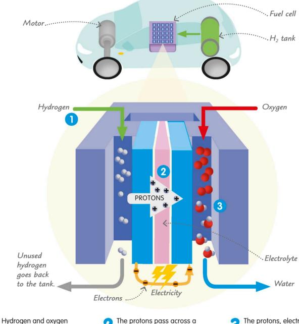
Hydrogen and oxygen enter the fuel cell. A chemical reaction takes place, and the hydrogen atoms split into protons and electrons. The protons pass across a chemical called an electrolyte, and the electrons flow through a wire, creating the electricity that powers the motor.
