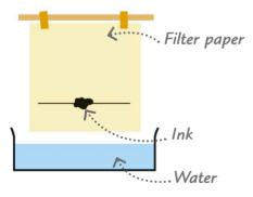
To separate the different dyes in black ink, a spot of ink is put on a sheet of filter paper, and the end of the paper is lowered into water.
