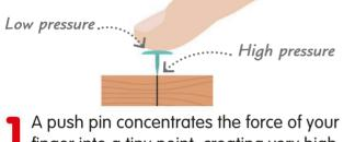
A push pin concentrates the force of your finger into a tiny point, creating very high pressure. The flat end spreads the pressure on your finger so it doesn't hurt.
