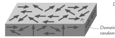
In materials that stick to magnets—such as iron—the electrons line up in clusters called domains, which act like mini magnets. However, the domains don't normally line up.
