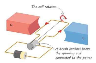
2 If the wire is twisted into a loop, the recoil force is upward on one side and downward on the other. This makes the loop spin around, provided it's loosely connected to the power source. This is an electric motor. Motors are used in everything from power tools to electric cars.
