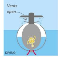
The ballast tanks are full of air so the submarine floats. Vents at the top of the ballast tanks are closed to keep the air trapped inside. 2 To dive, the submarine lets water into the ballast tanks and the vents open to let air out. This makes the submarine dense enough to sink.
