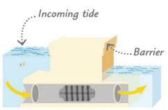
2 Tidal power and wave power both use the motion of seawater to drive turbines placed on the seabed. These power stations are expensive to build, but they can produce large amounts of electricity.
