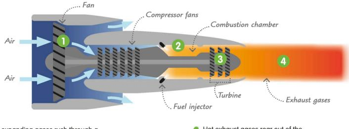
**3** The expanding gases rush through a fan called a turbine, spinning it around. This makes the fan and compressors at the front spin around too.
