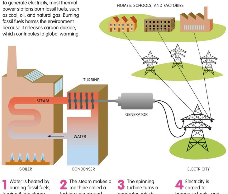
turning it into steam, which flows through a network of pipes.
