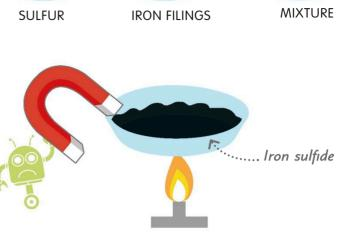
2 Iron sulfide compound If you heat iron and sulfur, a chemical reaction occurs, producing a black compound called iron sulfide. The iron and sulfur atoms are now chemically bonded and can't be separated with a magnet.
