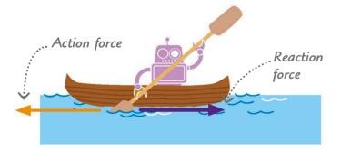
When you paddle in a canoe, pushing the water backward with the paddle creates an equal and opposite force that pushes the boat forward. The force pushing you forward is called the reaction force.
