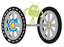
Multiplying distance When the effort is applied to the axle, the force applied by the wheel is reduced but the wheel moves much farther than the axle because it's bigger. This makes vehicles travel farther and faster.
