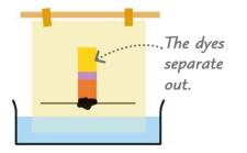
2 As the paper soaks up the water, the ink dissolves and travels with it. Different dye molecules travel at different speeds, so the colors separate out into horizontal bands.
