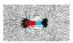
**1** A magnetic field is invisible, but you can see its effects by sprinkling iron filings over a bar magnet. The filings will align themselves along the lines of force.
