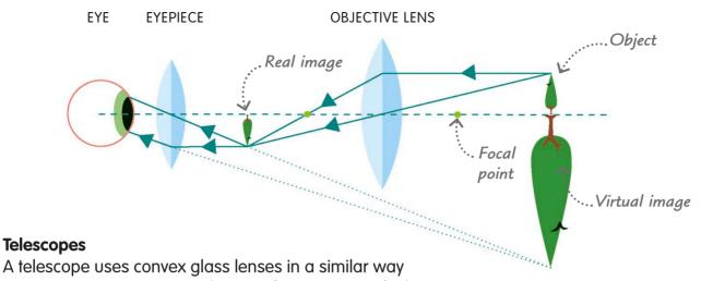
• A telescope uses convex glass lenses in a similar way to a microscope. However, a telescope forms a magnified image of a larger object that is far in the distance.
