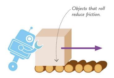
Objects that roll create less friction than objects that drag. That's why cars and bikes have wheels to move across the ground and bearings to help the wheels turn. However, wheels aren't completely friction-free—they still need enough friction to grip the ground and prevent a skid.
