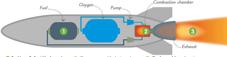
**1** Fuel (usually liquid hydrogen) and liquid oxygen are pumped from two large storage tanks to the engine. 2 The oxygen and fuel mix and burn in a combustion chamber. This creates a hot blast of exhaust gases from the back of the rocket. **3** The force of the exhaust gases rushing backward creates an equal and opposite force that pushes the rocket forward.
