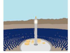
**5** Concentrated solar power stations use mirrors to focus sunlight onto a central furnace. It requires large areas of land and only works in places with sunny weather all year.
