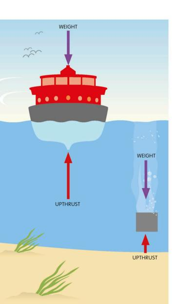
A solid block of steel will sink, but a steel ship of the same weight will float. The reason for the difference is that the ship contains a lot of air, so it weighs less per unit volume. We say it is less dense.
