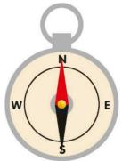
A compass is simply a magnetized needle balanced on a point. The needle lines up with Earth's magnetic field to show which way is north, helping you find your way.
