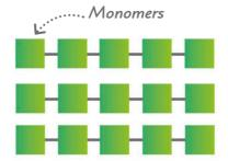
Thermoplastics can melt because they're made of separate polymer molecules that can slide over each other.
