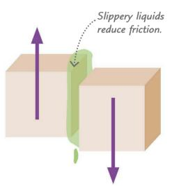
2 A great way to reduce friction between two objects is to put a layer of liquid between them. The liquid, called a lubricant, stops surfaces from snagging. The oil that cyclists put on bike chains is a lubricant. As well as helping the chain move smoothly, it protects the bike from wear.
