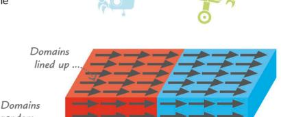
2 In a magnet, all the domains line up together. Their magnetic forces combine, creating a powerful magnetic force around the whole magnet.
