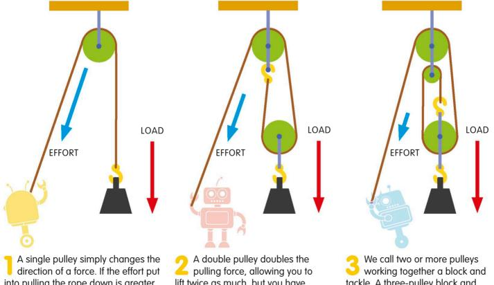
into pulling the rope down is greater than the load, the load rises.
