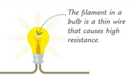
2 Resistance causes energy to be lost as heat or light. A very long, thin wire wound into a coil creates so much resistance that it will glow red or white hot. This is how electric heaters and filament light bulbs work.
