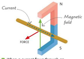
When a current flows through an existing magnetic field, the wire recoils (moves) in reaction because its own magnetic field is repelled by the magnet. This is called the motor effect.
