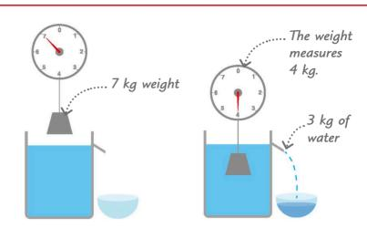
When this weight is out of the water, the weighing scales show its weight as 7 kg (70 newtons). 2 The weight displaces 3 kg of water as it's lowered, so the scales now show its weight as only 4 kg.
