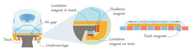
The Transrapid maglev system uses magnetic attraction to lift the base of the train's C-shaped undercarriage, creating an air gap between the train and track. 2 Guidance magnets in the train and the track use magnetic repulsion to stop the train from moving left or right and getting too close to the track. **3** The levitation magnets also drive the train. Computers switch them on and off rapidly to pull the train forward, slow it down, and keep it stable.
