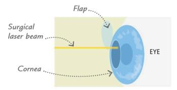
The precision of lasers makes them useful for delicate operations, such as laser eye surgery. A flap is cut in the eye's outer cornea, and a laser is fired in pulses to vaporize small areas of tissue, correcting near-sightedness. The flap is then folded back and allowed to heal.
