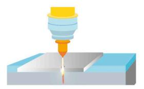
Some lasers produce powerful beams of 🕈 infrared light that can melt through metal, glass, plastic, and even diamond. Faster and more precise than electric drills, these lasers are used to make cooling holes in engines or the fine holes in shower heads, coffee makers, and food mincers.
