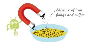
**1** Iron and sulfur mixture A mixture of iron filings and powdered sulfur is easy to separate with a magnet. The magnet
